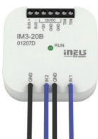
IM3-20B Binary input units
