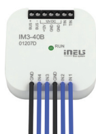
IM3-40B Binary input units
