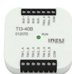
TI3-40B Temperature input, 4-channel
