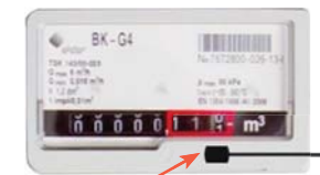
Built-in magnet in the gas meter
