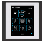
Hotel control unit with touch screen
