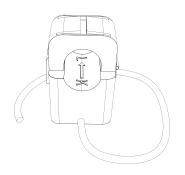
The arrow inside the current transformer CT50 must be directed to the appliance.
