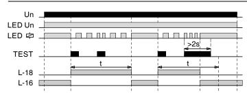
If the supply voltage is connected, the green LED Un lights up and at the same time the red LED indicates that the idle output contact "16" is closed. Pressing the TEST button on the device panel closes the output contact "18" and disconnects the phase wire "L" from the tested emergency lights.
