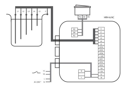
\* In case of HRH-6/DC, incoming supply is connected on terminals +Un and - Un.
