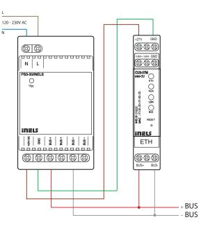
max. 32 units per BUS; max. 1A (PS3-30 / iNELS) per BUS
