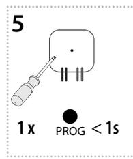
Press of programming button on actuator RFSA-61B shorter than 1 second will finish programming mode. The LED lights up according to the pre-set memory function.
