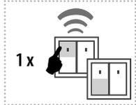
The output contact closes by pressing one button position, and opens by pressing the other button position.
