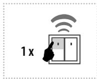
The output contact will be opened by pressing the button and closed after the set time interval has elapsed.
