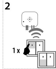
Pressing your chosen button on the RF transmitter assigns the function "close". The second position of the control "switch off" is assigned automatically (for 4-button in the same half of the RF transmitter).
