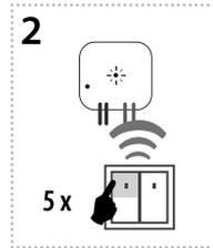
Assignment of the delayed off function is performed by five presses of the selected button on the RF transmitter (must be a lapse of 1s between individual presses).
