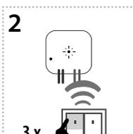
Three presses of your selected button on the RF transmitter assigns the function switch off (must be a lapse of 1 s between individual presses).
