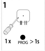
Press of programming button on actuator RFSA-11B for 1 second will activate actuator RFSA-11B into programming mode. LED is flashing in 1s interval.
