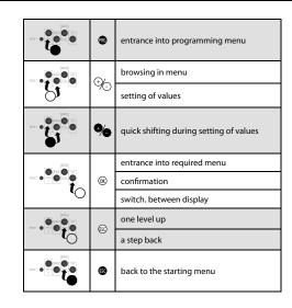
Device differs short and long button press. In the manual marked as:
